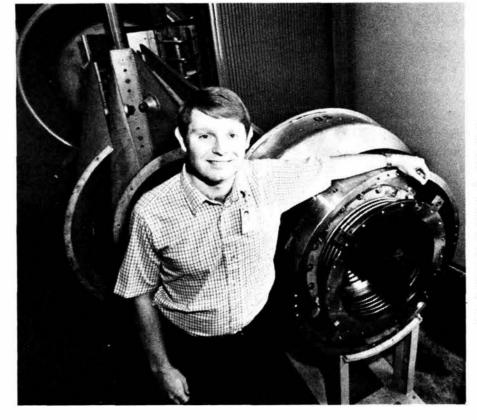
REGAN STINNETT (1261) is shown with the components of a PBFA module. The magnetically insulated transmission line of the module is a key component in the generation of negative ions. The technique was recently patented by DOE. Coinventors are Pace VanDevender (1260) and Bob Anderson (8354).
